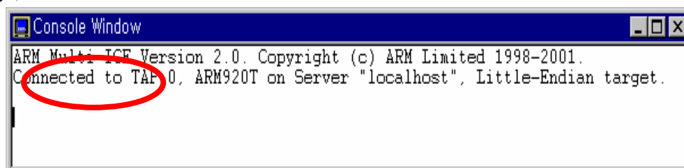
<Figure 2-10> ADW Console Window showing a successful connection with Multi-ICE
